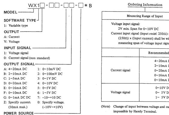
Recommended Range 4~20mA DC 2~10mA DC Current signal 0~20mA DC 0~16mA DC 0~10mA DC 0~10V DC Voltage signal 0~ 5V DC 1~ 5V DC
